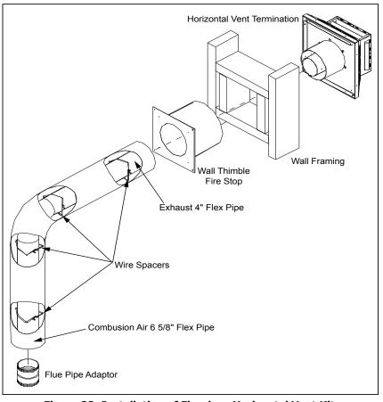
Figure 22: Installation of Fireplace Horizontal Vent Kit.
